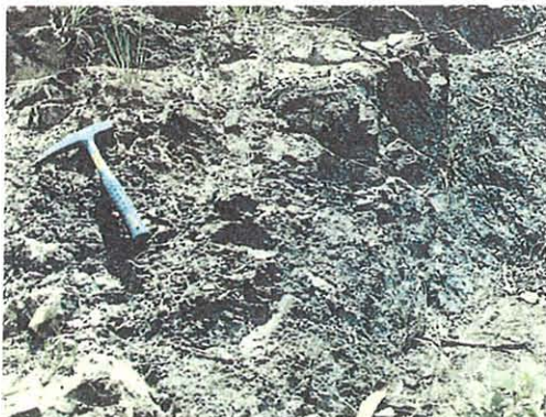
CLOSE UP OF BASALT (BA): Note lack of weathering in this exposure
